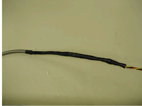
Figure XVIII: Waterproofing Reed Relay (Cont)
